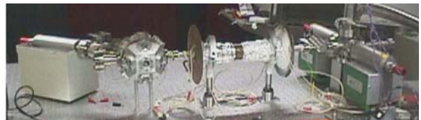
Figure 2: The cold atom source. From right to left: oven surrounded by two ion pumps, coils of the Zeeman slower (magnetic shield removed), capture region with an other ion pump in a magnetic shield. The total apparatus is one meter long.
